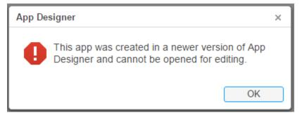
To enable editing of newer apps in a previous release, save the app in the release-specific format. Select **Save > Save Copy As** from any of the tabs in the toolstrip.
