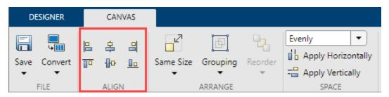
When you use an alignment tool, the selected components align to an anchor component. The anchor component is the last component selected, and it has a thicker selection border than the other components. To select a different anchor, hold down the **Ctrl** or **Shift** key and click the desired component twice (once to deselect the component, and a second time to select it again). For example,
